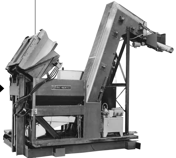
Magnetic belt conveyor and vibratory feeder system used to feed bearing races to heat treat furnace.
