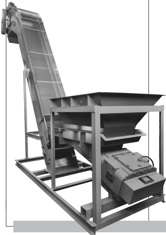
Magnetic belt conveyor and vibratory feeder system used to feed bearing races to heat treat furnace.
